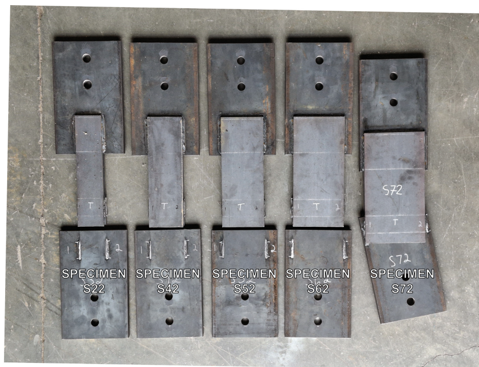
Fig. 13. Photograph of specimens that failed in the weld.
