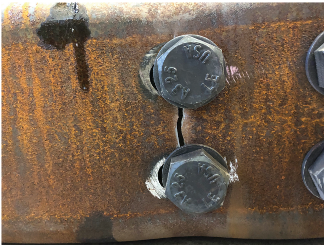
(c) Specimen 10 (HSS 12x8x3/8)
