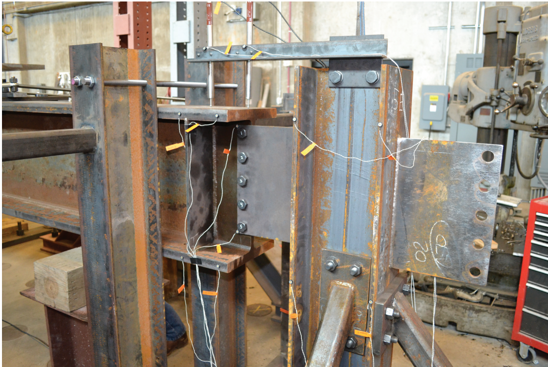
Fig. 5. Column and single-plate connection at beam end.
