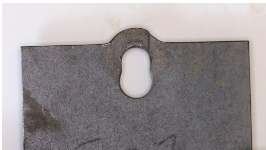
Fig. 3. Concentrically loaded specimen after testing.
