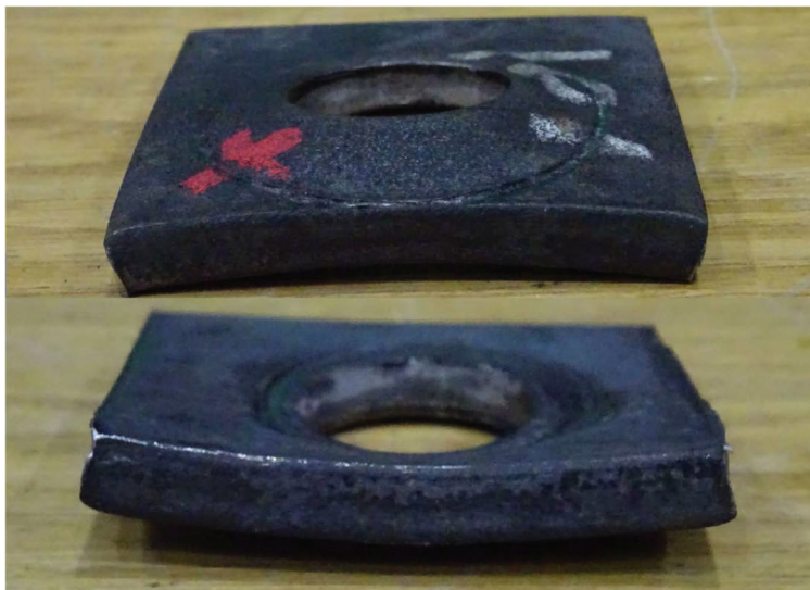
Fig. 10. 1/4 in. plate washer, offset orientation visual Category 2—likely failure.
