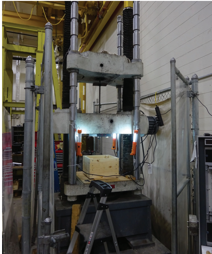
Fig. 2. Tinius Olsen Super-L universal testing apparatus.
