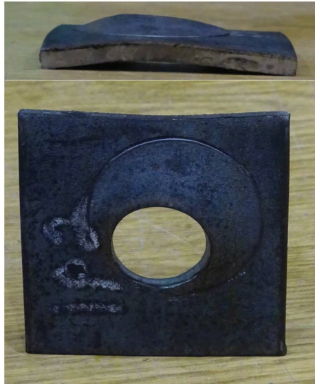
Fig. 11. 1/4 in. plate washer, offset orientation visual Category 3—clear failure.
