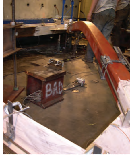
(b) Large out-of-plane deformation
