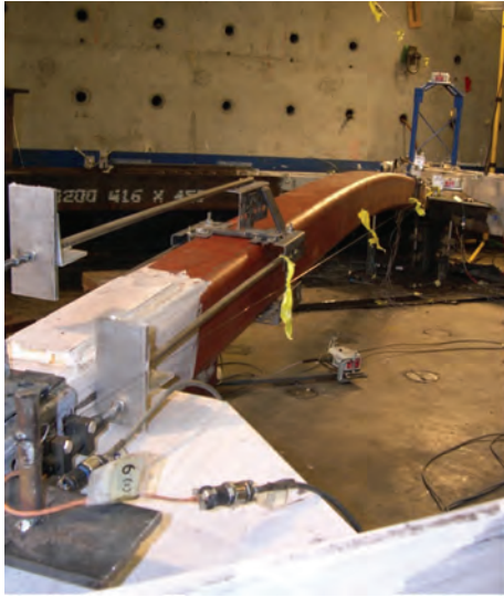
(a) Initial brace buckling
