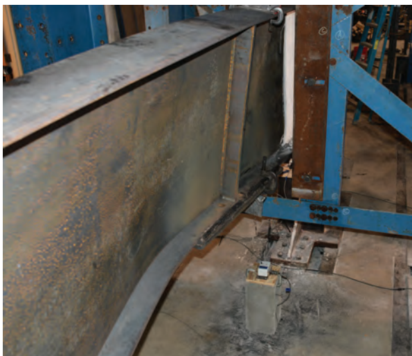
Fig. 10. Lateral torsional buckling of the beam of Specimen 4E-1.5-1.75-36a.
