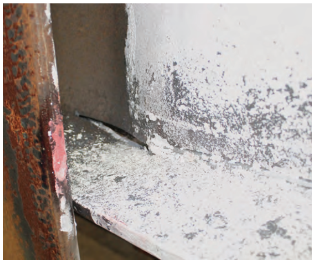
Fig. 13. Fracture of beam web to beam flange weld of Specimen 4E-1.5-1.75-36b.
