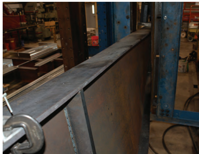
Fig. 10. Lateral torsional buckling of the beam of Specimen 4E-1.5-1.75-36a.
