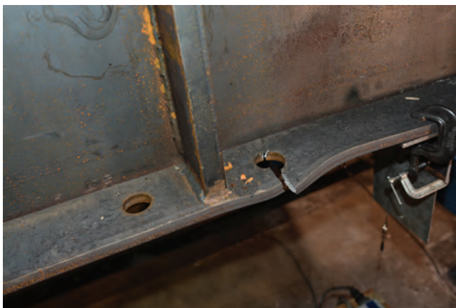
Fig. 8. Bottom flange fracture at bolt holes of Specimen 4E-1.5-1.75-36a.
