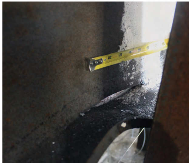
Fig. 13. Fracture of beam web to beam flange weld of Specimen 4E-1.5-1.75-36b.
