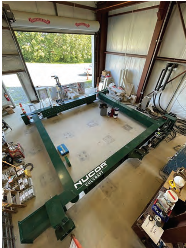
Fig. 5. Cantilever diaphragm testing rig at UMass Amherst.
