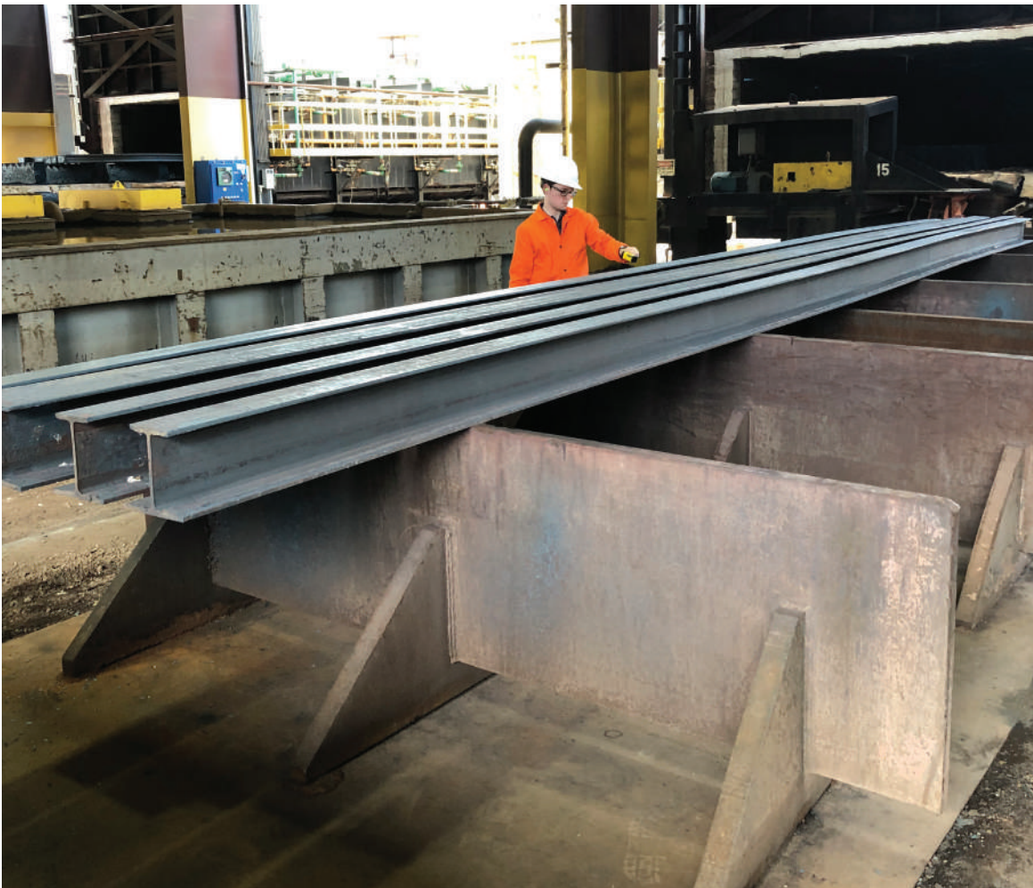
Fig. 3. Noncontact temperature measurements being taken of the cooling A-shapes.
