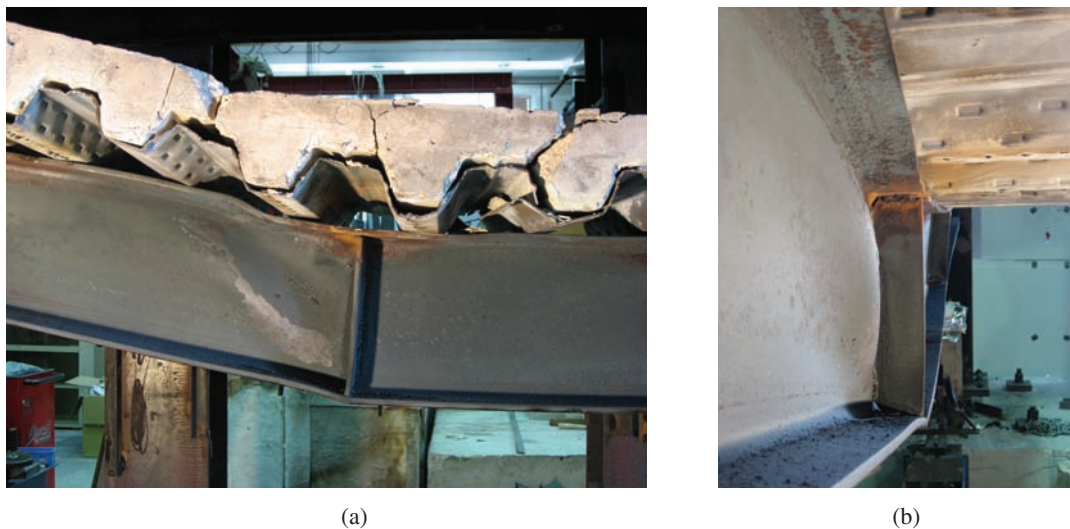
Fig. 22. Shear buckling of the beam web near the load points.
