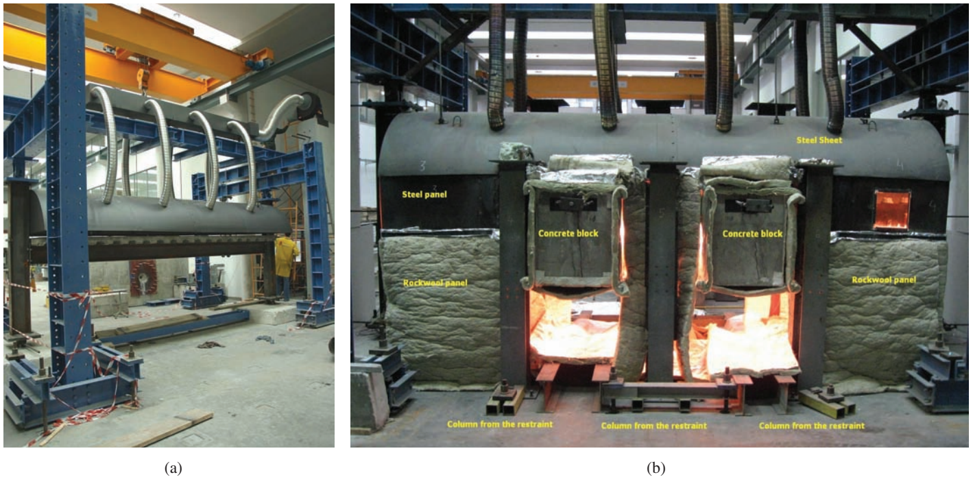
Fig. 4. General layout: (a) preparation; (b) during a fire test.
