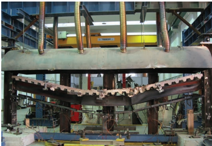
Fig. 14. Deformed structure after test FJ01.
