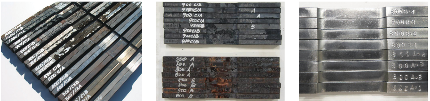
Fig. 5. Coupons before and after cleaning.
