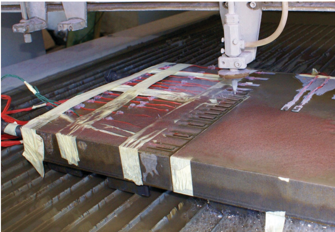
Fig. 8. Sectioning of the flange plate by water-jet cutting. (Photograph courtesy of Professor Darko Beg)
