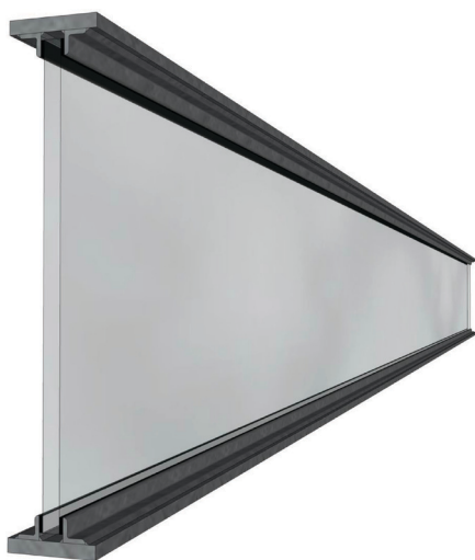
Fig. 4. Hybrid steel-glass beam with adhesive web-to-flange connections. (Figure courtesy of Professor Frantisek Wald)
