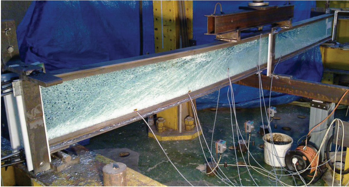
Fig. 5. Full-scale test of a steel-glass beam. (Photograph courtesy of Professor Frantisek Wald)
