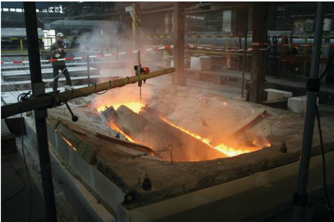
Fig. 2. Collapsed composite slab assembly during fire test. (Photograph courtesy of Professor Frantisek Wald)
