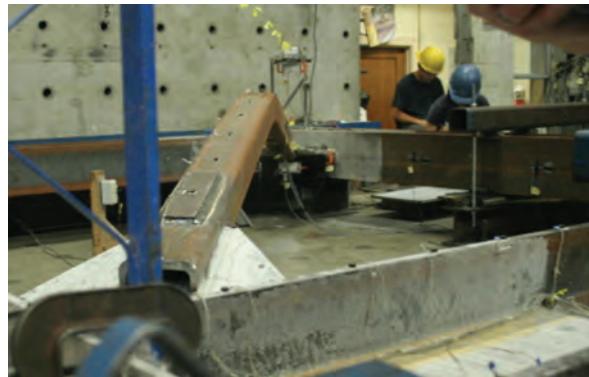
(c) Buckled brace just prior to connection weld fracture
