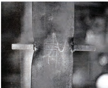
Fig. 1. Web local yielding failure in a full-width plate-to-HSS connection, with plates in compression.
