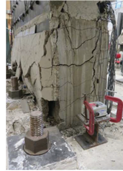
(b) Side view RC wall portion
