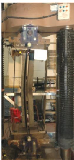
(a) Experimental and analytical shape (showing von Mises stress)
