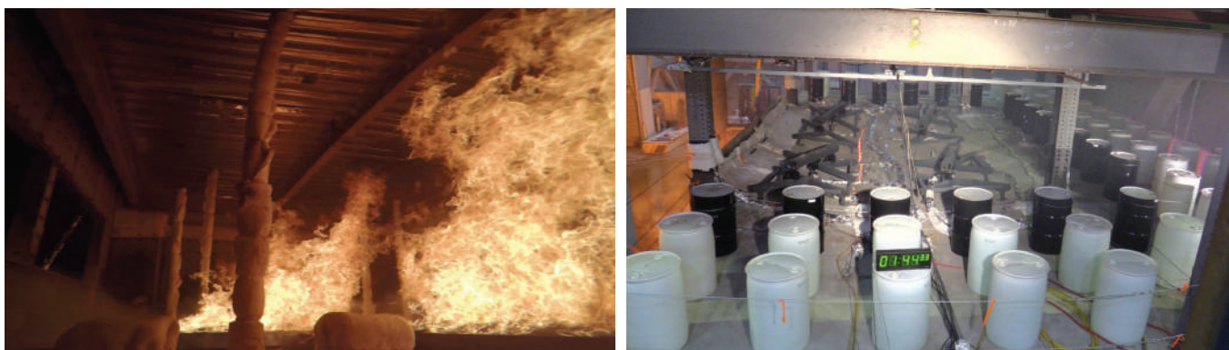
Fig. 1. (a) Compartment fires with natural gas burners and (b) floor loading.
