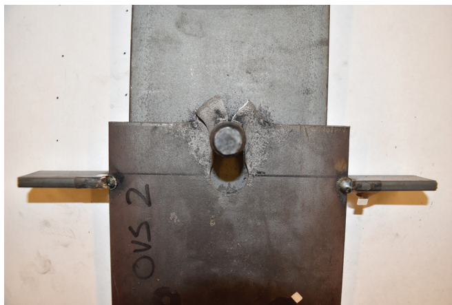
(a) Specimen OVS2 after testing
