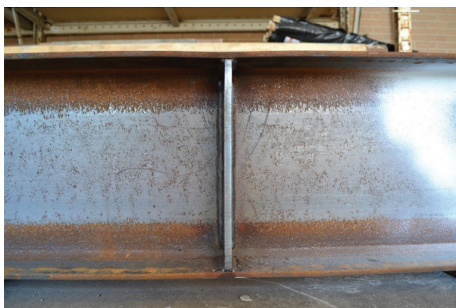
Fig. 13. Elevation view of W12×26 DC-E0 after testing.
