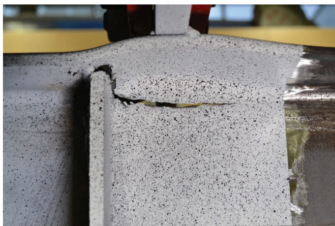
Fig. 14. W12x26 ST-E2 after testing with weld and web fracture.
