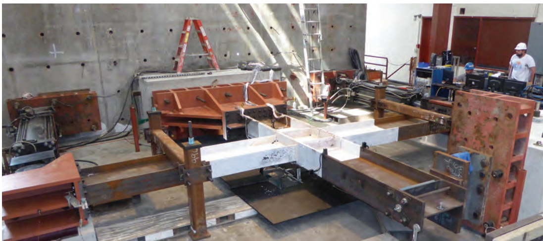
Fig. 2. Interior moment connection test setup.
