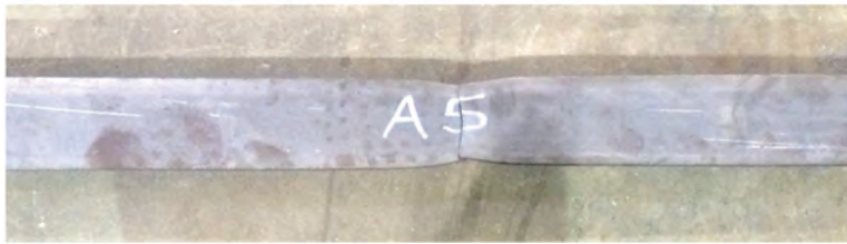
Fig. 9. Typical gross section fracture.
