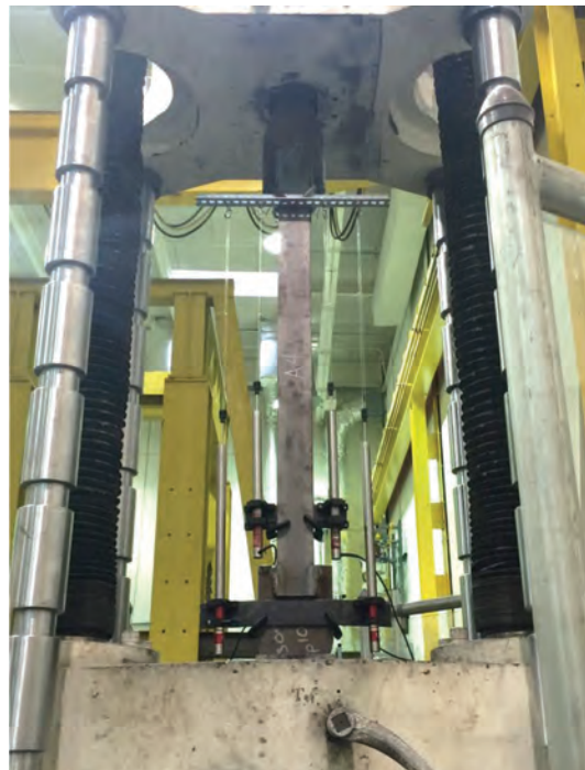
Fig. 8. Experimental setup of tension specimen.
