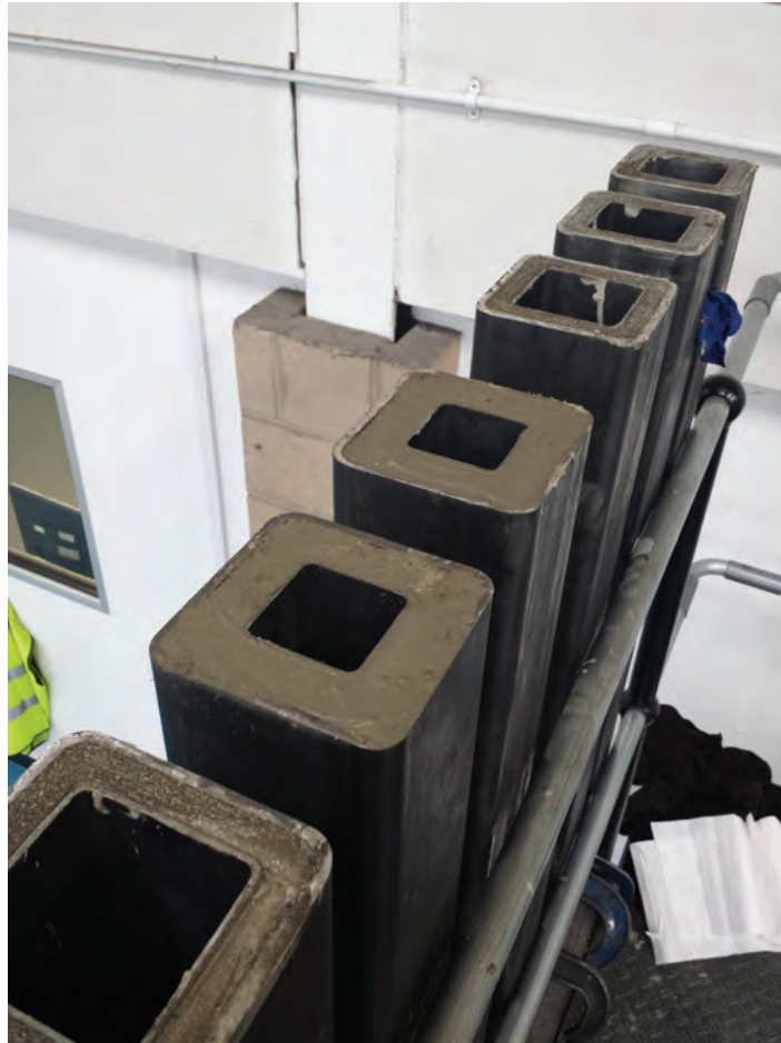
Fig. 9. CFDST test specimens under fabrication.
