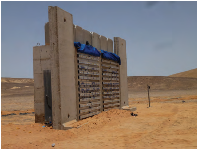
(a) HSS test specimens in concrete reaction structure
