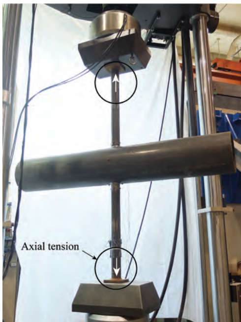
Fig. 2. Testing arrangement for round-to-round HSS cross-connections.
