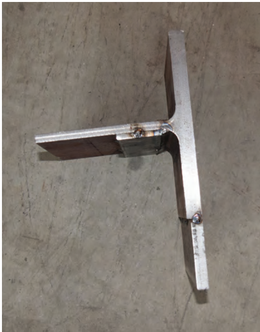
Fig. 14. Doubler plate specimens: (a) \frac{3}{4} -in. specimen; (b) \frac{1}{4} -in. specimen.
