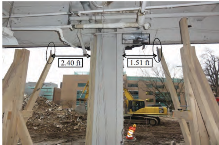
Fig. 6. Vertical LVDT to the south (in circle on left) and north (in circle on right) of the removed column and horizontal LVDT (rectangle) attached to the removed column.
