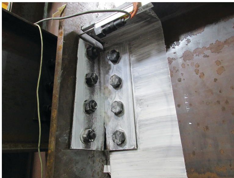
Fig. 5. Tearing in double-angle connection in specimen BS-BB at 9% story drift.
