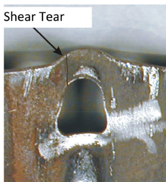
Fig. 3. A downstream bolt failing in shear tearout (Cai and Driver, 2010).
