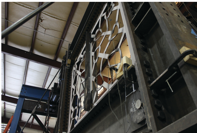
Fig. 8. Global shear buckling in fifth-story RS-SPSW specimen.
