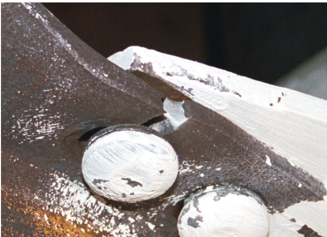
Fig. 1. Initial fracture in the beam flange of connection test FS-07.
