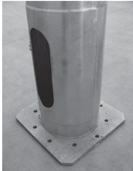
Fig. 3. Base section of as-built test specimen (note doubler plate around hand-hole detail).
