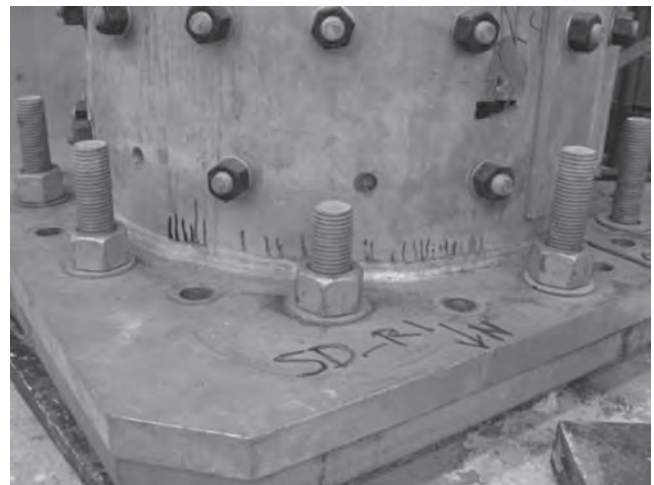
Fig. 12. Specimen TR_1: north crack at upper weld toe after inspection with dye penetrant.
