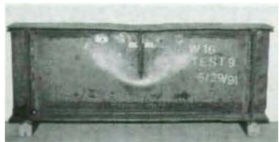
Fig. 5. Failure mode 1—web crippling below stiffeners (test 9).
