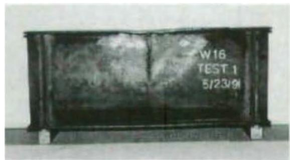
Fig. 7. Failure mode 2—local stiffener crippling (test 1).
