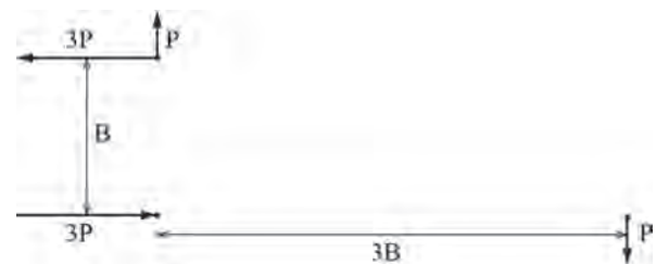
Fig. 2. Illustration of Maxwell's theorem using a 3:1 cantilever.
