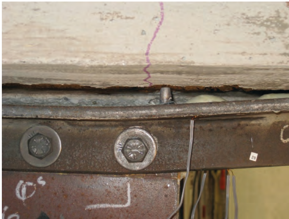
Fig. 20. Specimen FOB: rupture of stud connectors near the end of the top chord.
