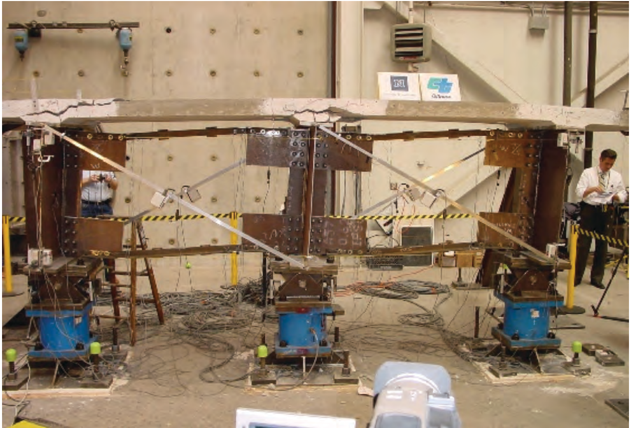
Fig. 14. Specimen F0A: deformation and damage at 5% drift.
