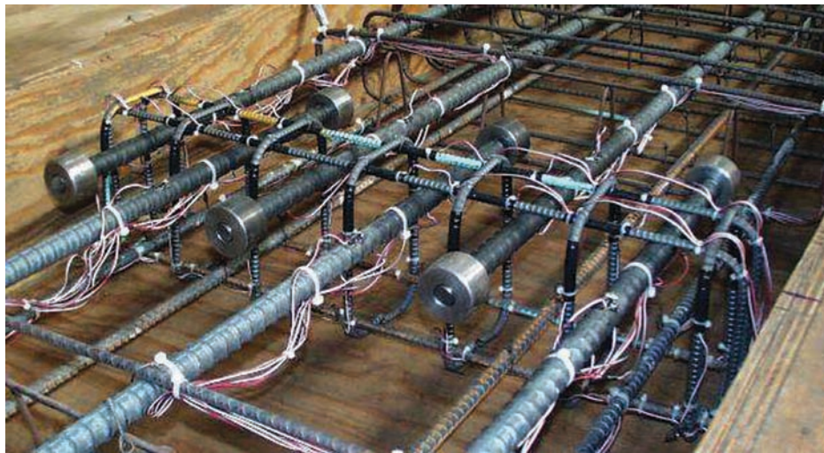
Fig. 23. Headed bar detail.
