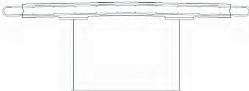
Fig. 14. Single (interior) box girder and deck unit.
