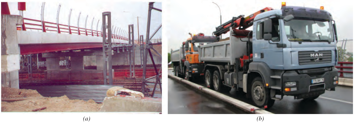
Fig. 7. (a) Tested bridge; (b) loading of bridge (photographs courtesy of Professors Mohammed Hjiij and Alain Lachal).
