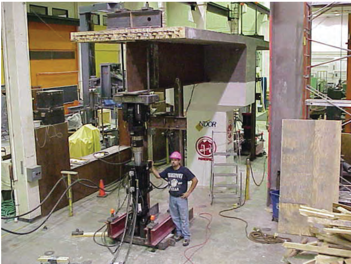
Fig. 6. Specimen 1 cycling test setup and fixtures.
