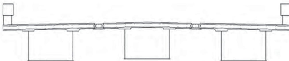
Fig. 15. Three adjacent box-girder units.
