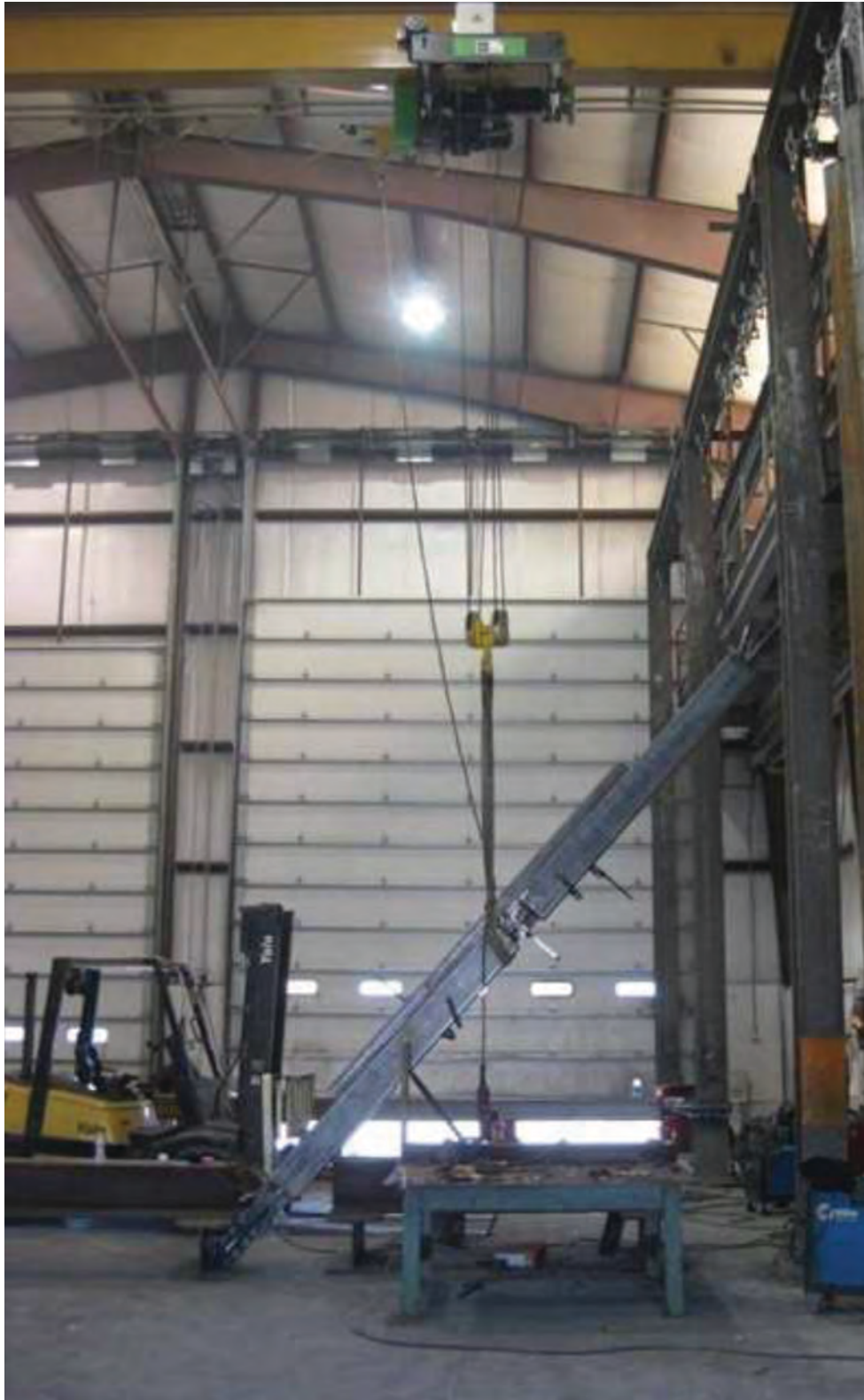
Fig. 11. Prototype spliced in inclined position.
