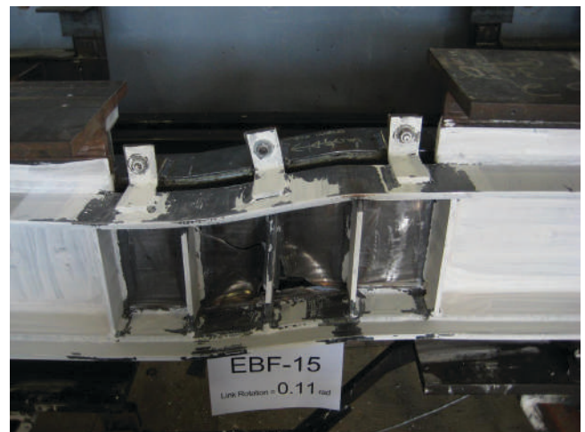
Fig. 7. Replaceable eccentrically braced link at 0.11 rad of rotation (photograph courtesy of Professor C. Christopoulos).
