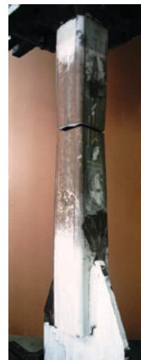
Fig. 13. Various slotted connections and failure modes for HSS bracing members (illustrations courtesy of Professor Robert Tremblay).
