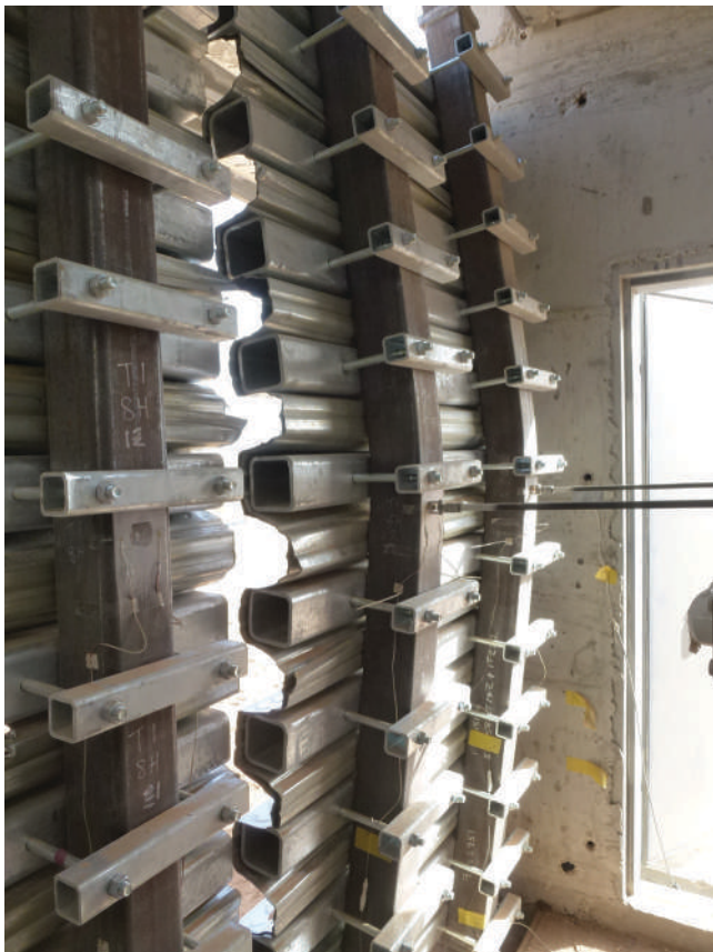
Fig. 1. HSS structural wall assembly after testing (photograph courtesy of Professor J. A. Packer).
