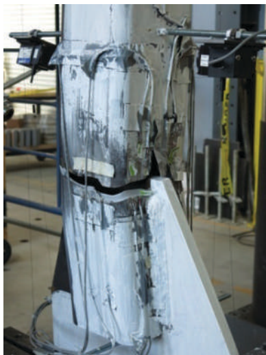
Fig. 13. Various slotted connections and failure modes for HSS bracing members (illustrations courtesy of Professor Robert Tremblay).
