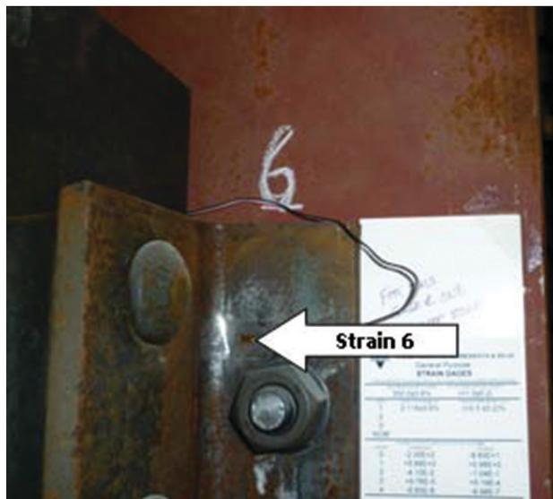
Fig. 11. WC250 strain gauges.
