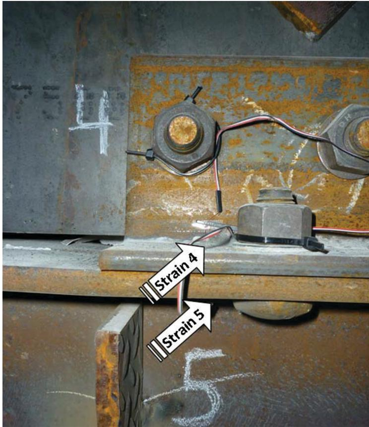
Fig. 10. WC250 strain gauges.
