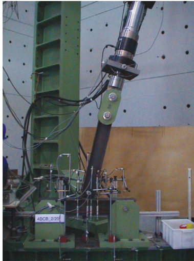
Fig. 16. Test on beam-to-column connection under combined axial and shear forces (figures courtesy of Professors Nadia Baldassino and Riccardo Zandonini).
