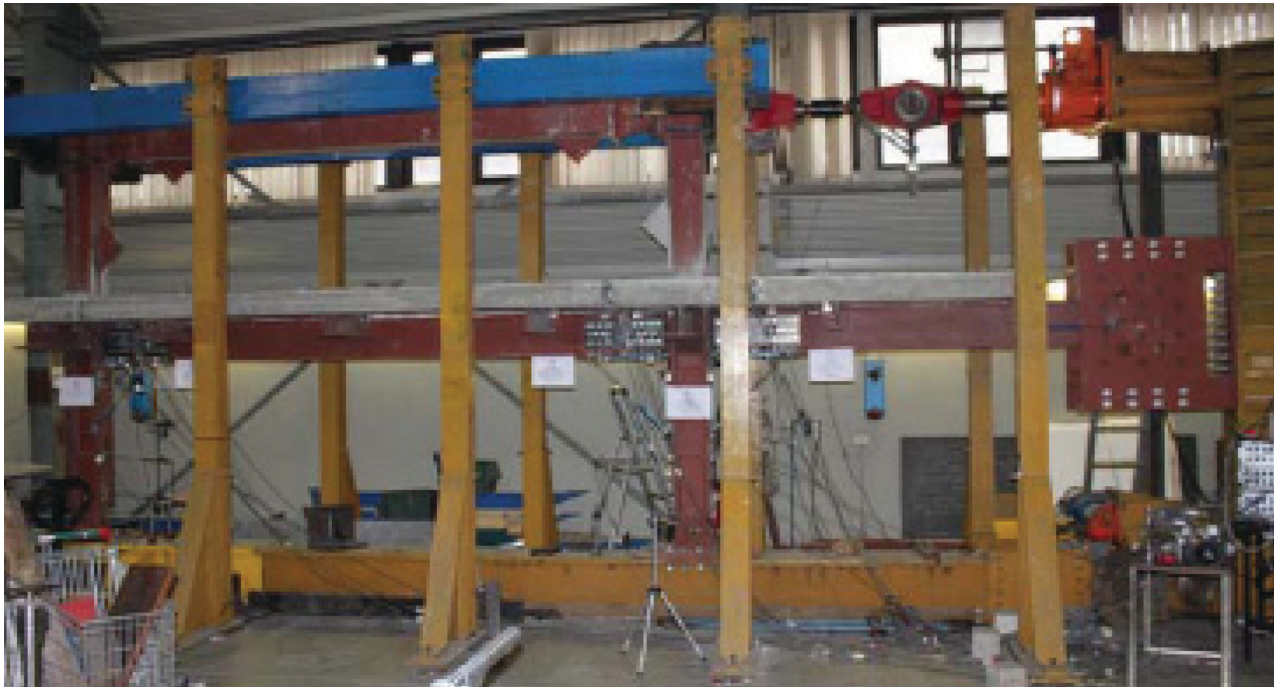
Fig. 3. Full-scale test frame with FUSEISI devices and failure mode (photo courtesy of Professor Carlo Castiglioni).
