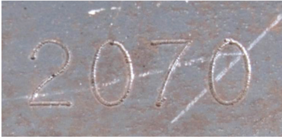
Fig. 3. Piece marking made with impact stylus system.
