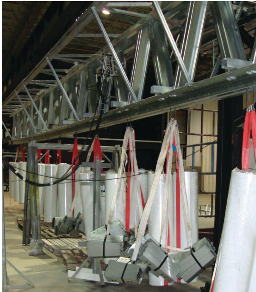
Fig. 4. Cold-formed trussed beam under full-scale load test (beam span 20 m = 67 ft). (Photo courtesy of Professor Eduardo Batista)
