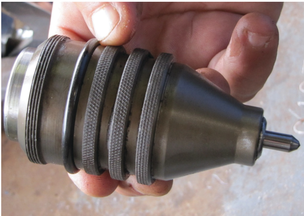
Fig. 5. Stylus used to mark specimen.
