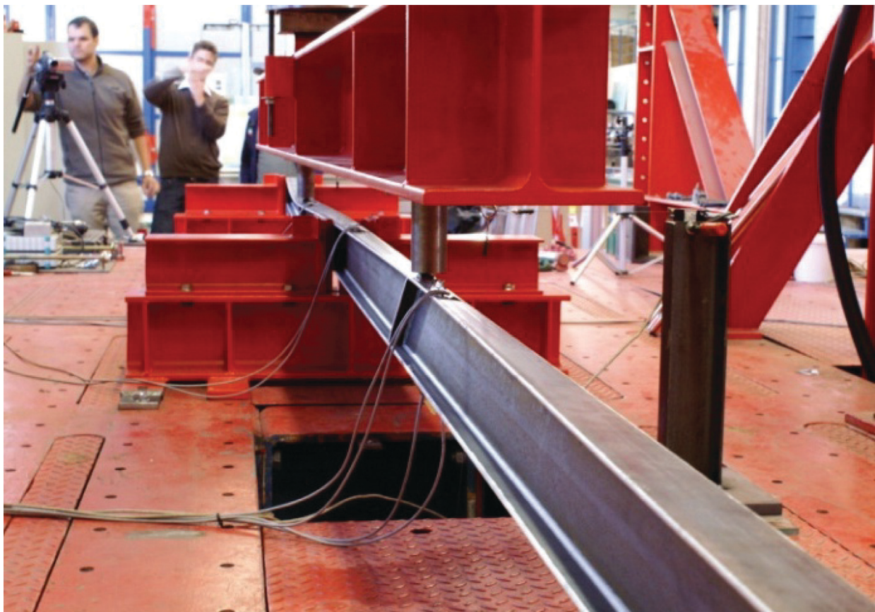
Fig. 1. Lateral buckling test. (Photo courtesy of Professor Markus Feldmann)
