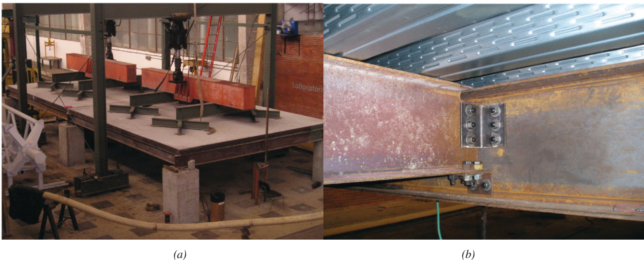
Fig. 6. Full-scale testing of a semi-continuous floor system and one of the connections. (Photo courtesy of Professor Eduardo Batista)
