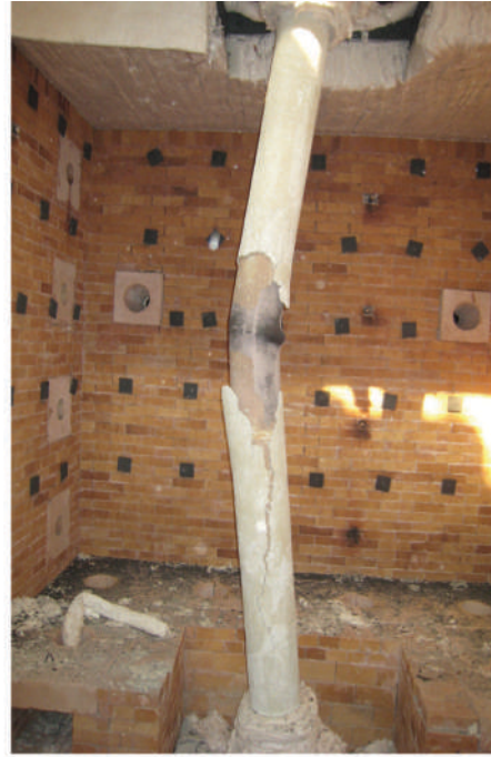
Fig. 8. Fire testing of ultra-high-strength composite columns: (a) test assembly; (b) failure of composite column. (Figure courtesy of Professor Richard Liew)
