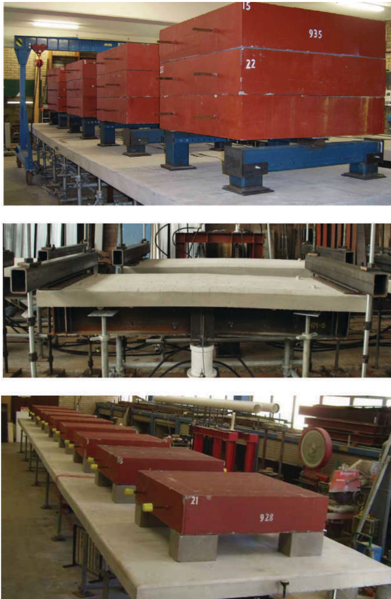
Fig. 6. Long-term tests with simple beam, simple beam with a negative moment and continuous beam. (Figures courtesy of Professor Gianluca Ranzi)
