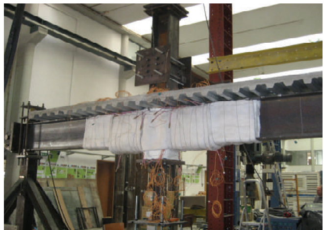
Fig. 2. Fire testing of a full-scale beam-to-column connection. (Figure courtesy of Professor Luis da Silva)
