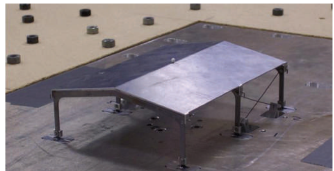
Fig. 3. Wind tunnel model with three frames, showing longitudinally braced bay.
