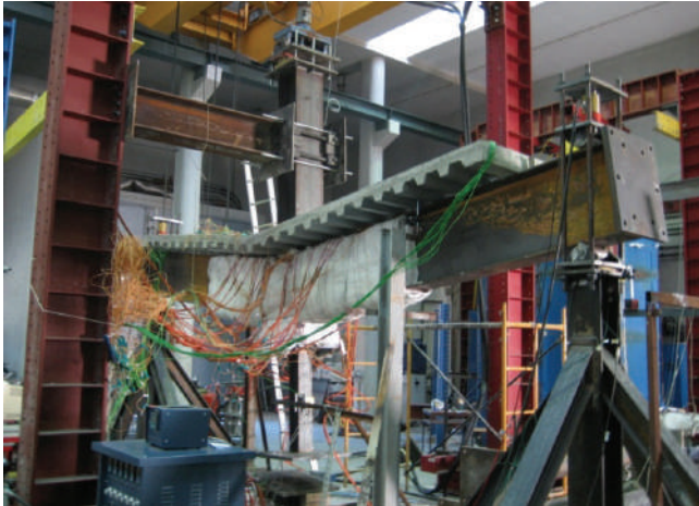
Fig. 3. Fire testing of a structural composite subassemblage. (Figure courtesy of Professor Luis da Silva)
