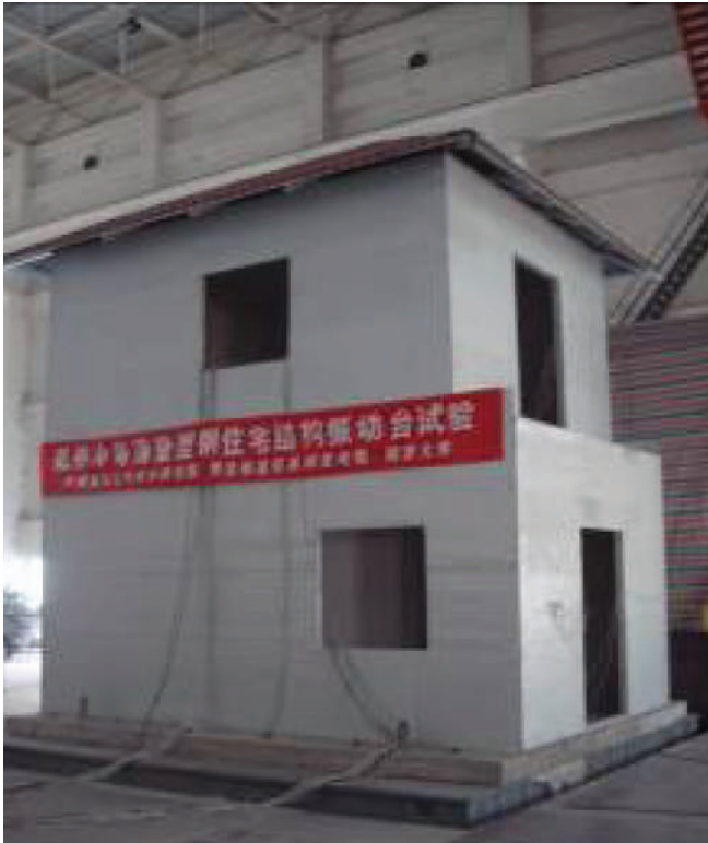
Fig. 7. Full-scale two-story building to be tested on shaking table. (Photo courtesy of Professors Z.-Y. Shen and Y.-Q. Li)
