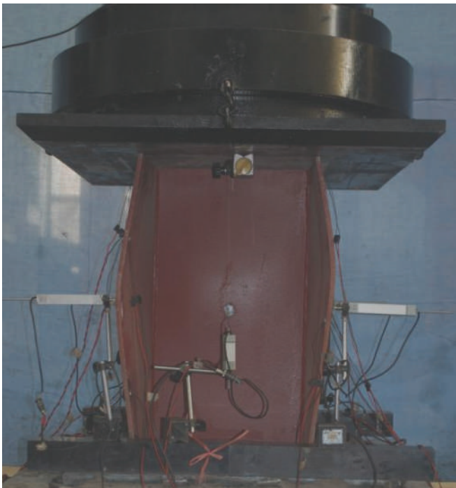
Fig. 3. Stub-column test of shape with slender web and flange elements in 65-ksi yield stress steel. (Photo courtesy of Professor Gang Shi)
