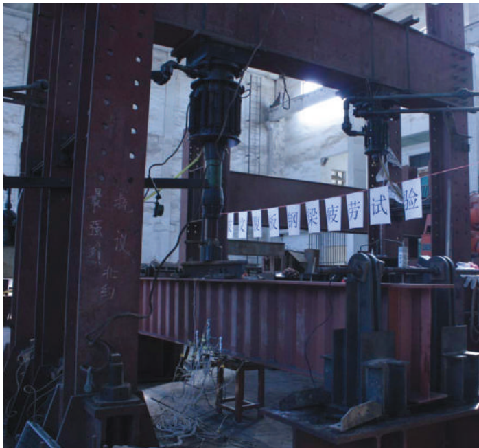
Fig. 6. Testing of girder with trapezoidal corrugated web. (Photo courtesy of Professor G.-Q. Li)
