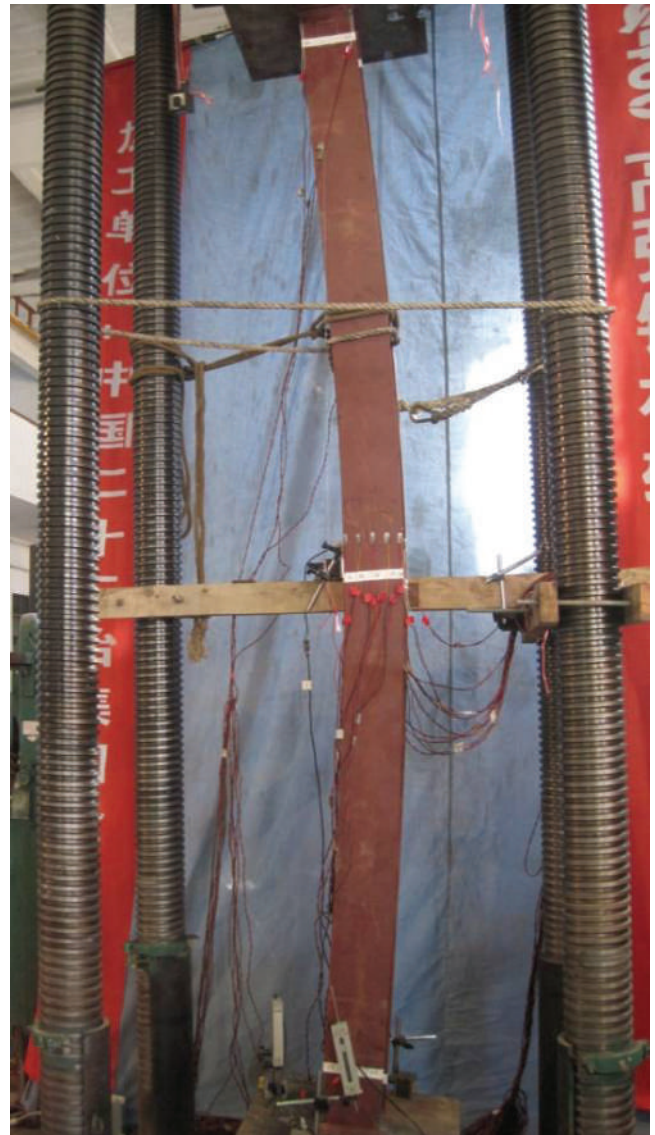
Fig. 4. Long column test of welded built-up shape in 65-ksi yield stress steel. (Photo courtesy of Professor Gang Shi)
