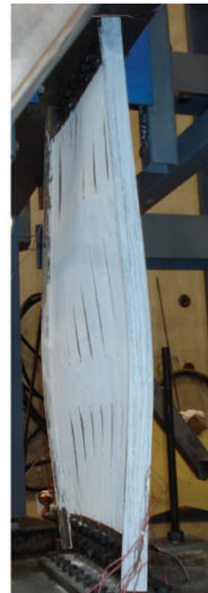
Fig. 5. Global lateral-torsional buckling of an SSP.
