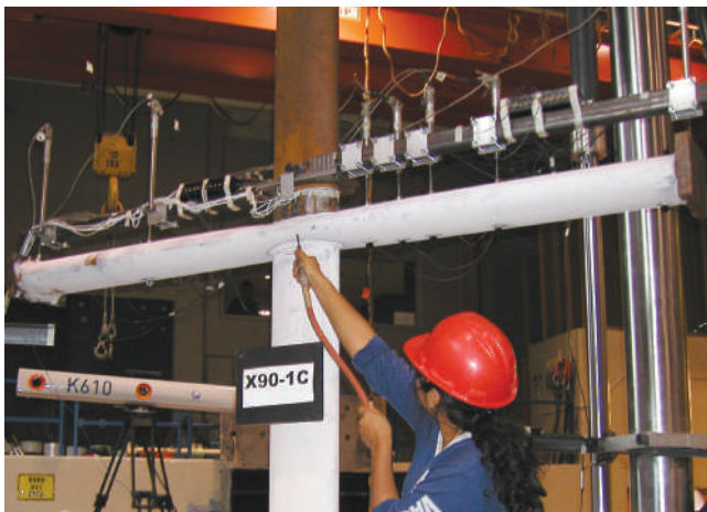
Fig. 1. Test of an elliptical HSS connection (courtesy of Professor J.A. Packer).
