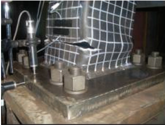
Fig. 1. Typical damage at column base that eventually led to frame collapse. (Photo courtesy of Professor M. Nakashima)
