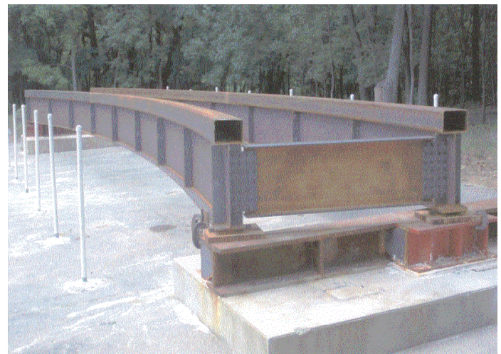
Fig. 6. Test specimen for a two-thirds scale curved tubular flange bridge structure (Courtesy of Professor Richard Sause).
