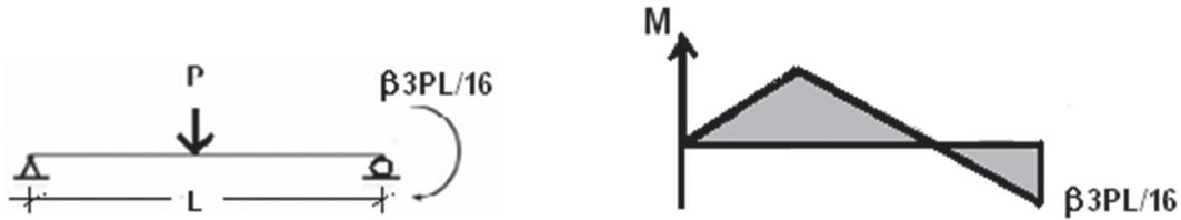
Type 6—Concentrated Load with Pinned Ends
