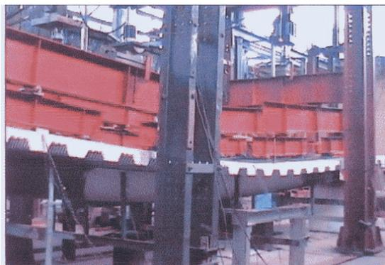
Fig. 5. Full-scale composite beam test with deep trapezoidal steel deck (Photo courtesy of Professor Mark Bradford).
