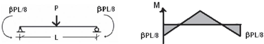
Type 5—Mid-span Concentrated Load with One End Moment
