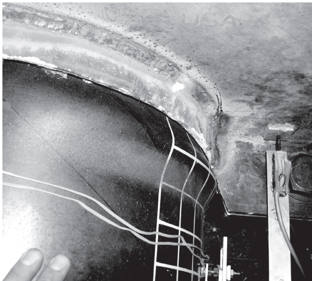
Fig. 7. Photos of behaviors noted in the CFT tests: (a) local buckling; (b) tears developing at the peak of the bulge.
