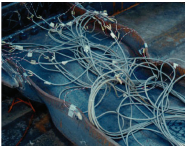
Fig. 9. Photograph of hinge formation at the end of testing specimen HH-9.
