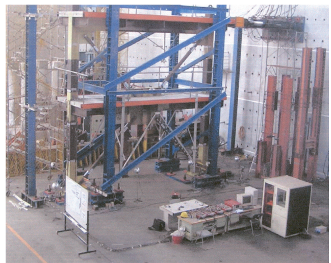
Fig. 3. Two-story SCBF with a two-story X-brace configuration (photo courtesy of Charles W. Roeder).
