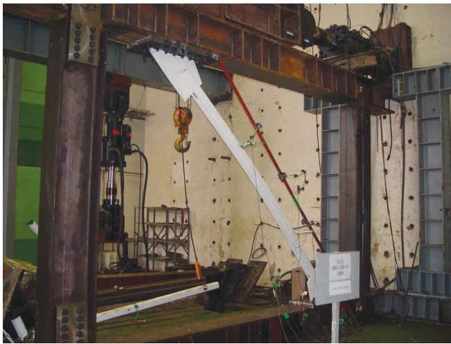
(a) Overall buckling (-0.375%).
