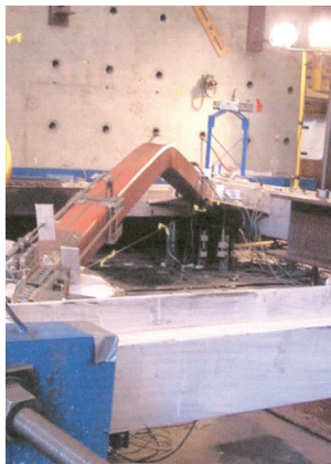
Fig. 2. Post-buckling deformations in the SCBF test frame brace and gusset plate (photo courtesy of Charles W. Roeder).
