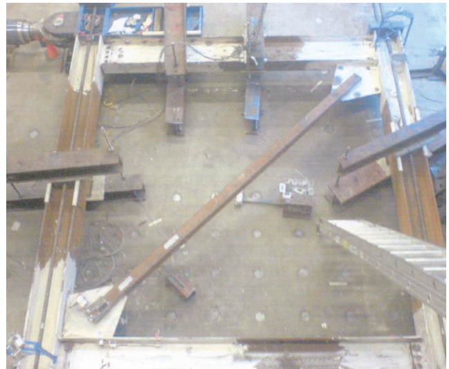
Fig. 1. Single-story SCBF test specimen (photo courtesy of Charles W. Roeder).
