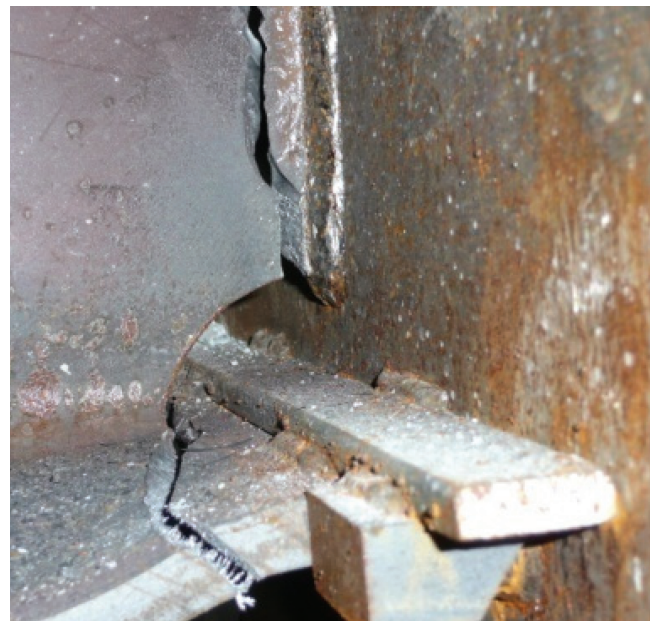
Fig. 2. Failure mode of older beam-to-column connection. (Photo courtesy of Professor M. Nakashima)
