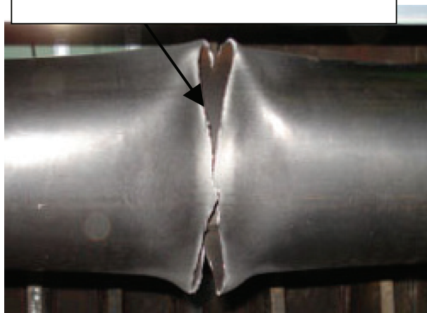
(a) Development of crack
