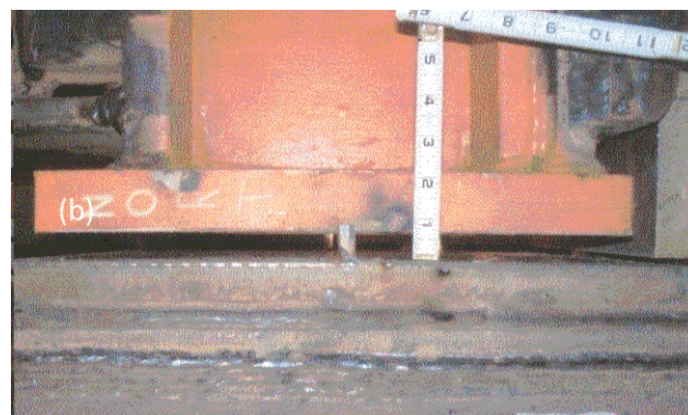
Fig. 8. Rocking displacement at the base of a column of the SC-CBF (Courtesy of Professors James M. Ricles and Richard Sause).
