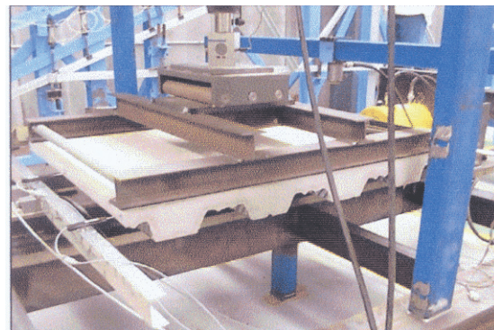
Fig. 3. Push-test for stud shear connector performance (Photo courtesy of Professor Mark Bradford).
